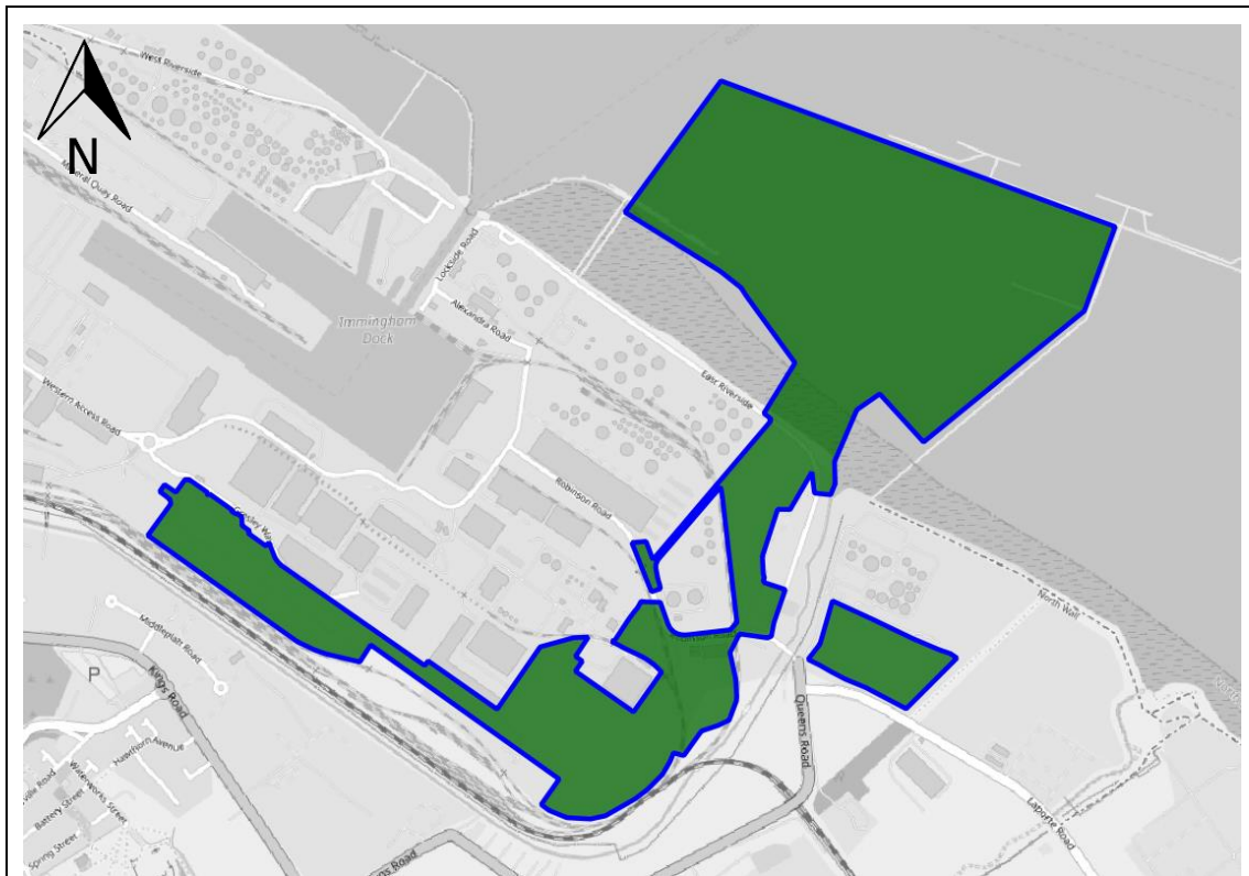
Figure 6 UXO hazard zone plan of the Site
